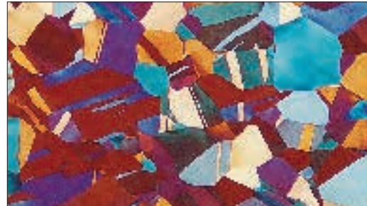
Alpha grains containing annealing twins in phosphorous-deoxidized arsenical bronze that was annealed and lightly cold drawn (Klemm's I reagent, polarized light, 50X).
