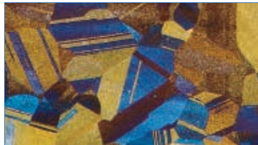
Equiaxed grain structure of Elgiloy (Co – 20% Cr – 15% Fe – 15% Ni – 7% Mo – 2% Mn – 0.15% C – 0.05% Be) after hot rolling and annealing revealing annealing twins (Beraha's reagent, crossed polarized light plus sensitive tint, 100X).
